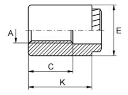
Female thread A = M2,5 Height K = 13 Hole diameter +0.1 = 4.2 Min distance to edge = 2.4 Min material thickness = 1.5 Outer diameter E = 6 Thread length = 9
